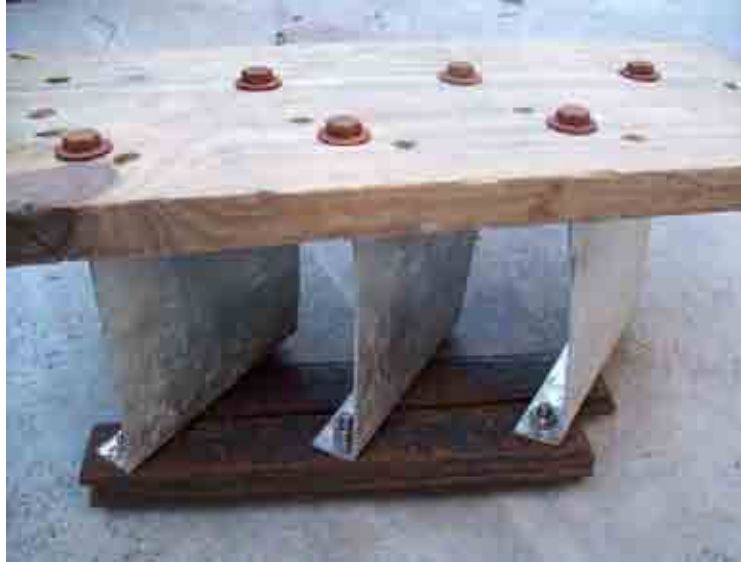
Figure 11: The towed device with 400g weights attached to the lower surface of the keels
