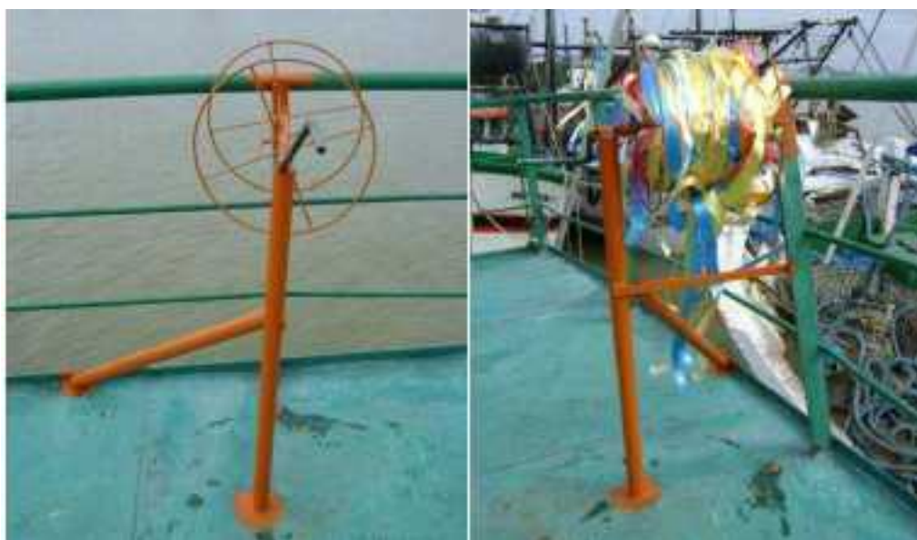
Figure 4. Toriline's hauling device in the FV Akira V .
