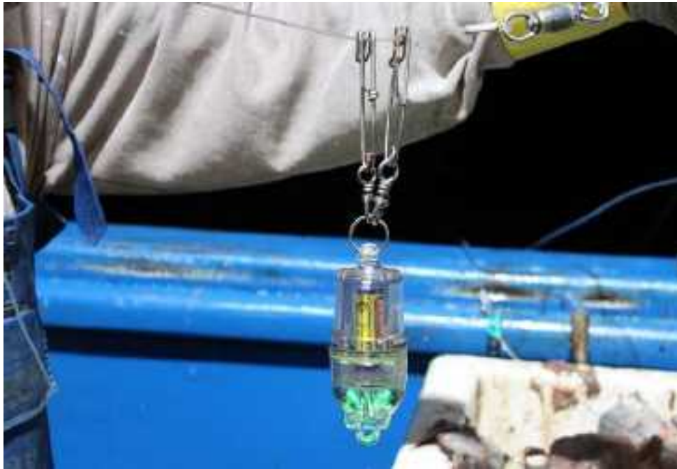
Figure 2. Electric fishing light attached to a branch line just above the 75 g leaded swivels.
